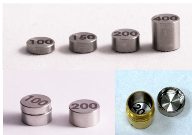
Figure 1 Selection of solid references and combining them to achieve the required volumes.
